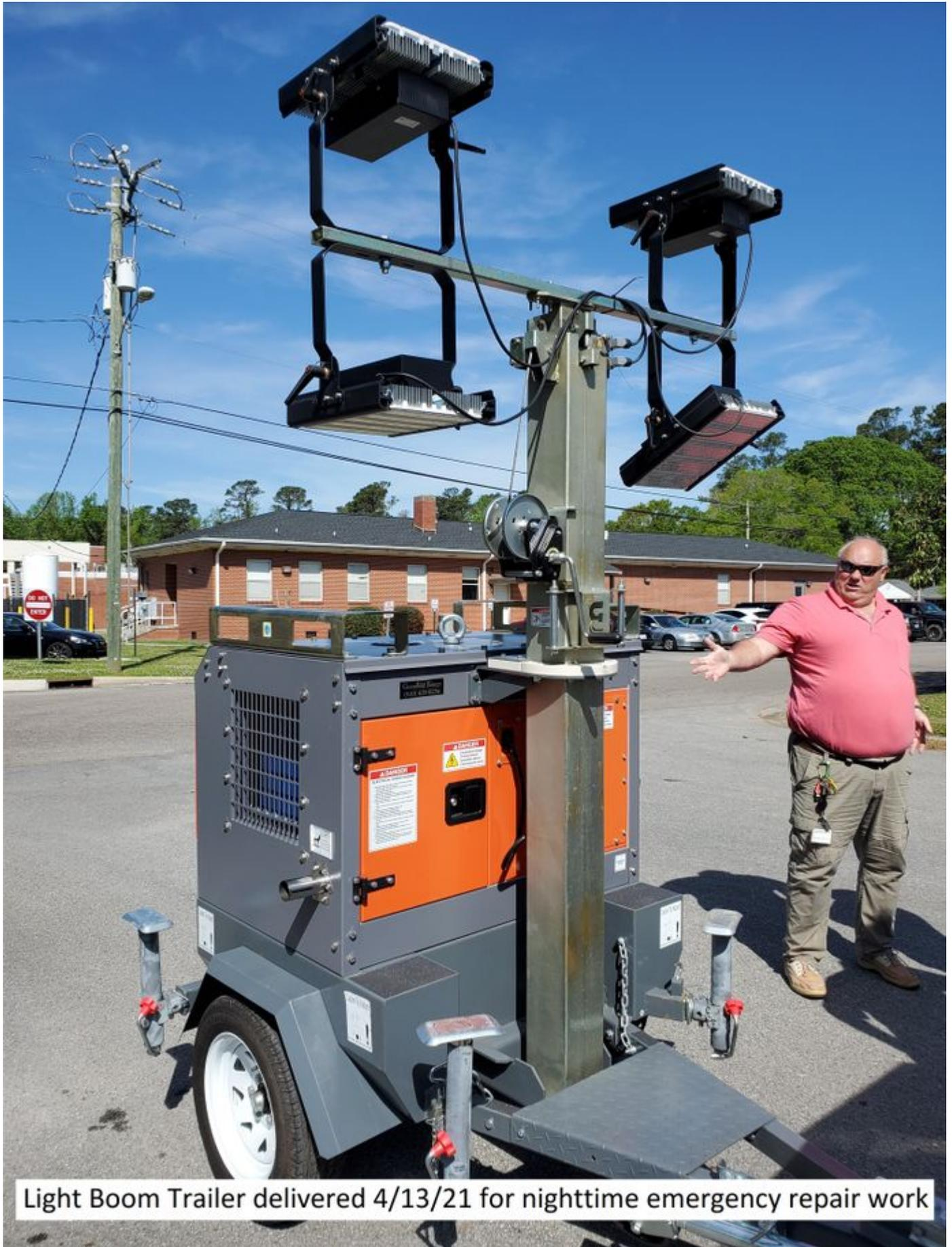
Light Boom Trailer delivered 4/13/21 for nighttime emergency repair work
